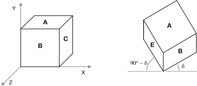
11. What is the name of the projection on the left side of the figure, knowing that the object is a cube?
