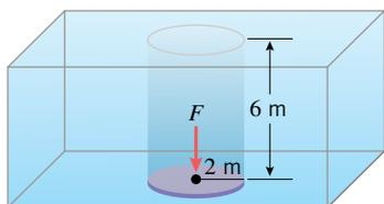
The fluid force is the fluid pressure times the area.
