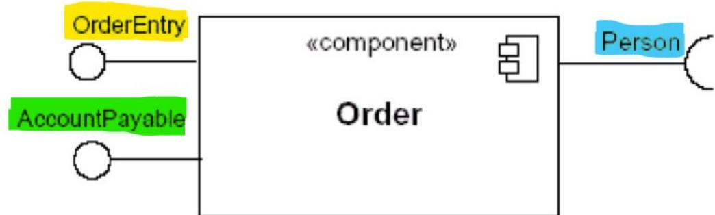
A connector can link multiple providers and customers that share the same provided and required interface
