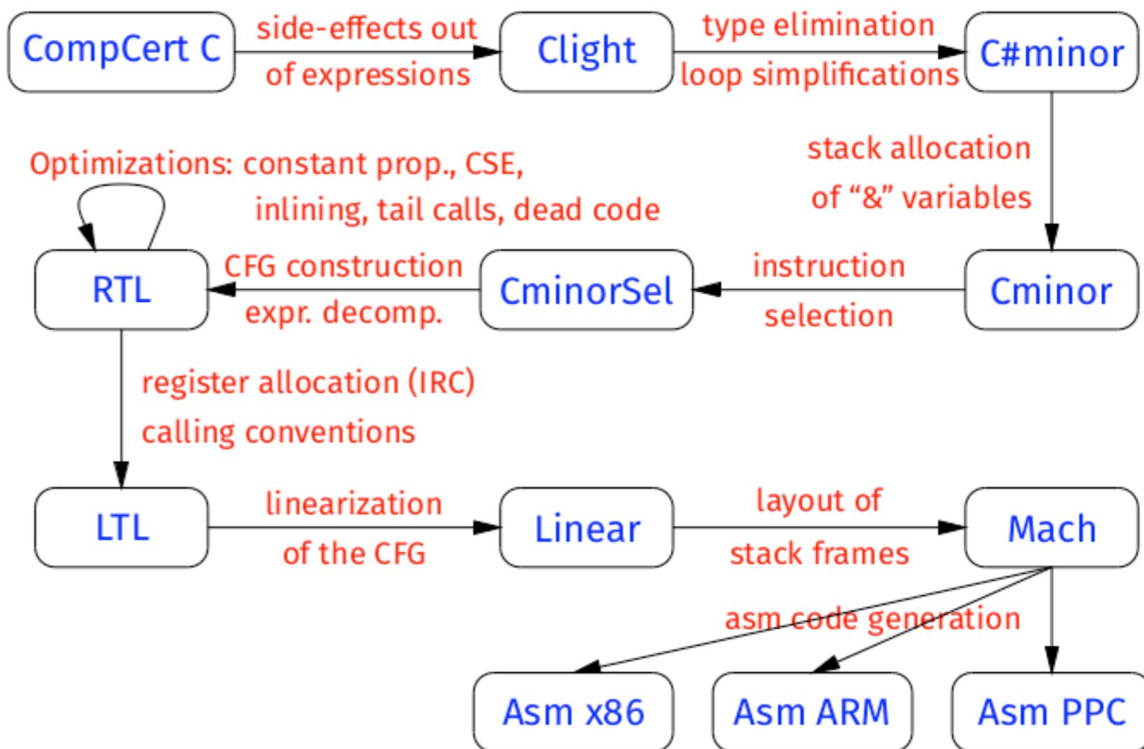
**Part 2: Compilation of CompCert C AST to assembly AST.** This part is the bulk of the compiler and the one that is proved correct in Coq. It is structured in 16 passes and uses 10 intermediate language, as depicted on the following diagram.
