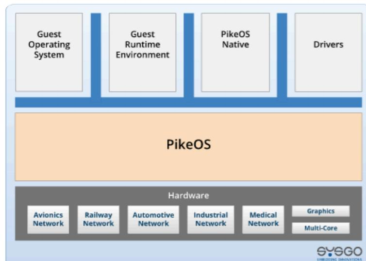
Due to its separation kernel approach, PikeOS is the first choice for systems which demand protection against Cyber-Security attacks. In addition to the broad usage within millions of IoT and edge systems, it has also been deployed within various high critical communication infrastructures.
