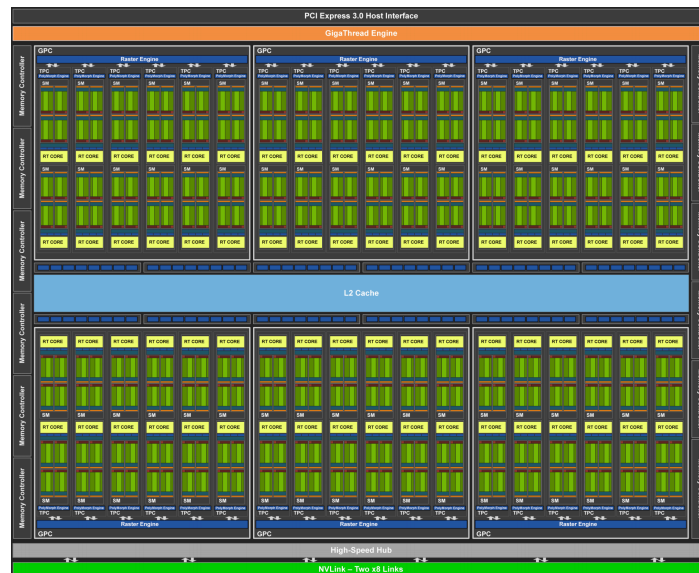
Fig. 12.4.8: NVIDIA Turing Architecture (image courtesy of NVIDIA)
