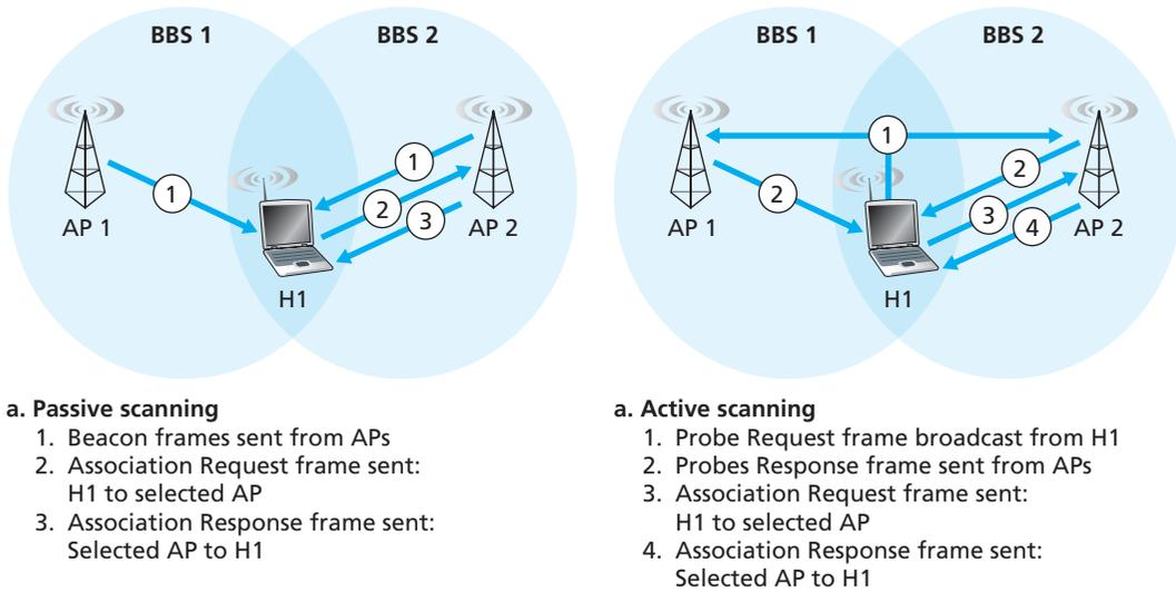
**Figure 6.9** ♦ Active and passive scanning for access points
