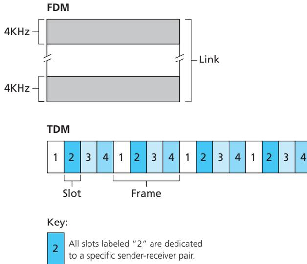
**Figure 5.9** ♦ A four-node TDM and FDM example
