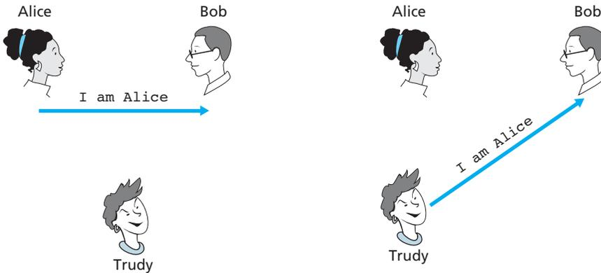
**Figure 8.15** ♦ Protocol *ap1.0* and a failure scenario
