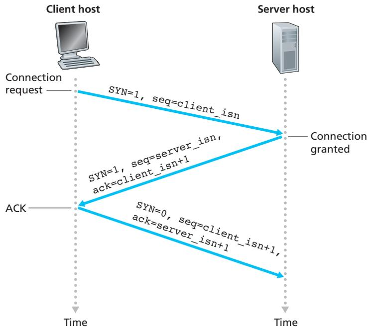
**Figure 3.39** ♦ TCP three-way handshake: segment exchange
