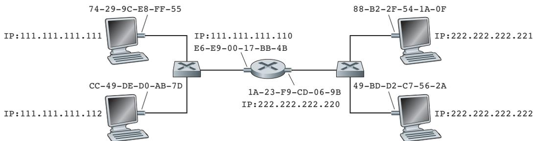
**Figure 5.19** ♦ Two subnets interconnected by a router
