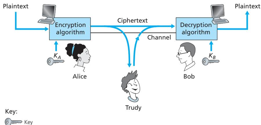
**Figure 8.2** ♦ Cryptographic components
