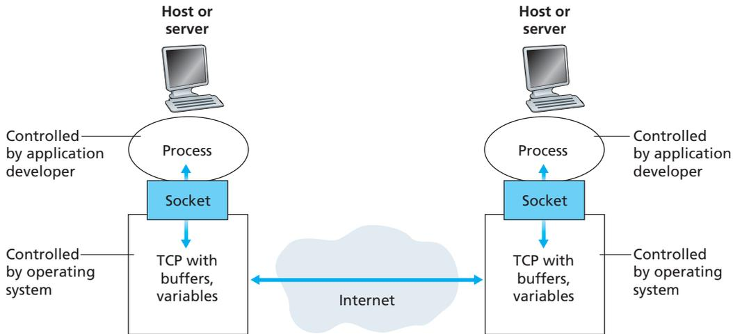
**Figure 2.3** ♦ Application processes, sockets, and underlying transport protocol
