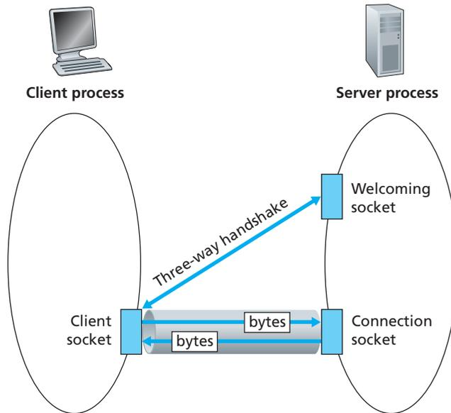
**Figure 2.29** ♦ The TCPServer process has two sockets
