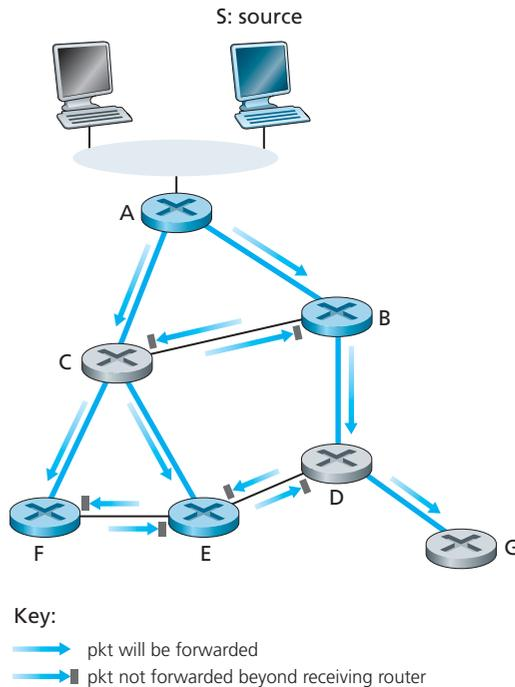
**Figure 4.50** ♦ Reverse path forwarding, the multicast case
