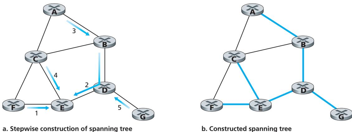
Figure 4.46 ♦ Center-based construction of a spanning tree
