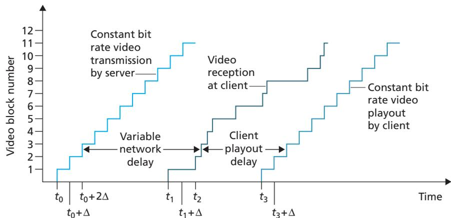
**Figure 7.1** ♦ Client playback delay in video streaming
