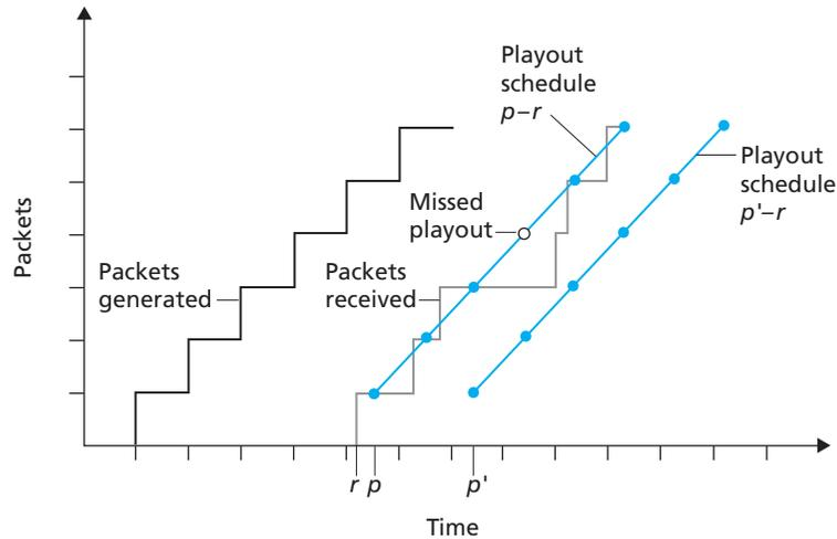
**Figure 7.7** ♦ Packet loss for different fixed playout delays
