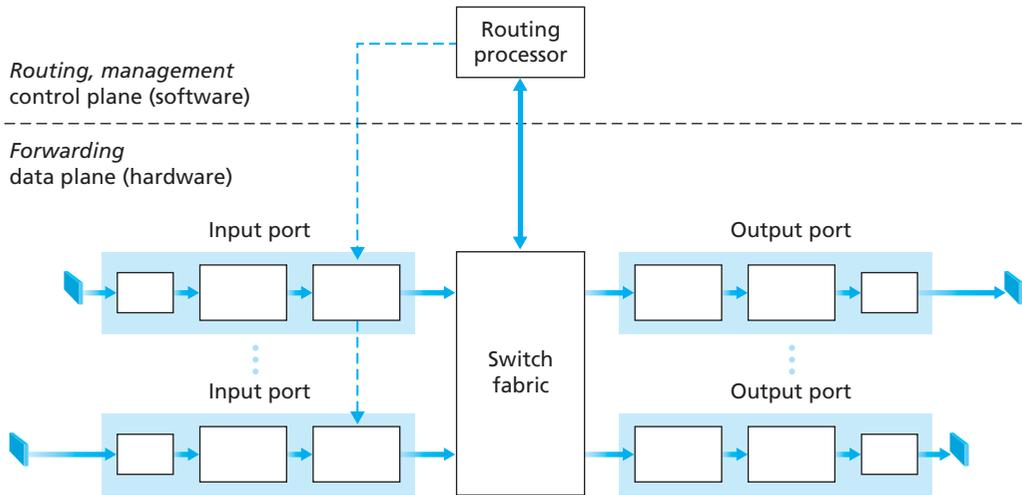
**Figure 4.6** ♦ Router architecture
