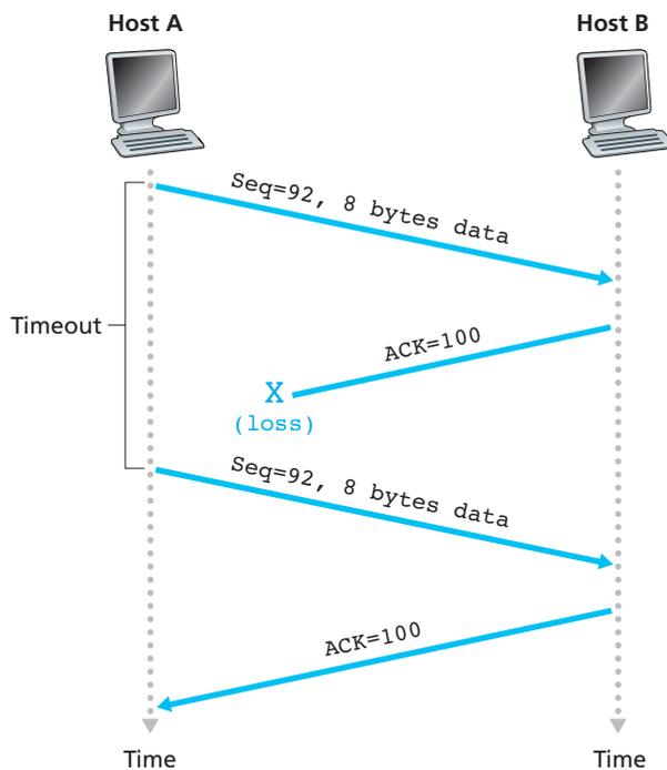
**Figure 3.34** ♦ Retransmission due to a lost acknowledgment
