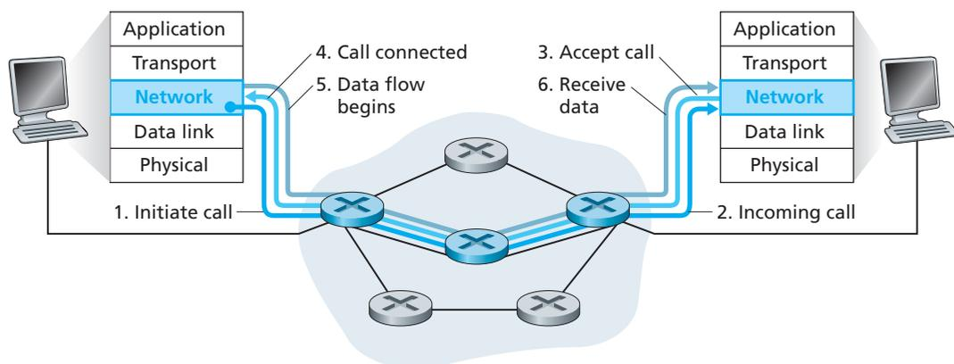
**Figure 4.4** ♦ Virtual-circuit setup
