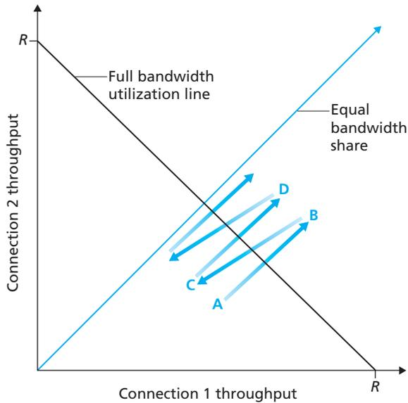
**Figure 3.56** ♦ Throughput realized by TCP connections 1 and 2
