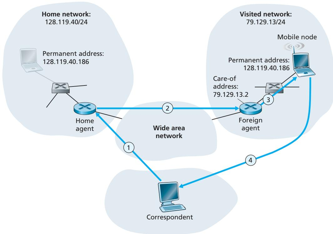
**Figure 6.23** ♦ Indirect routing to a mobile node
