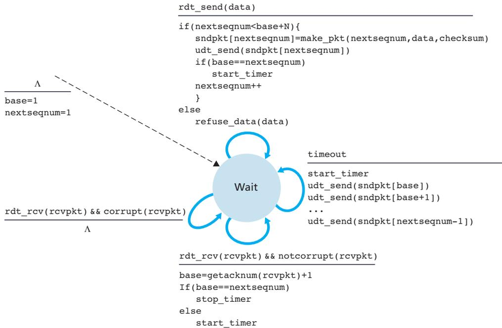
**Figure 3.20** ♦ Extended FSM description of GBN sender
