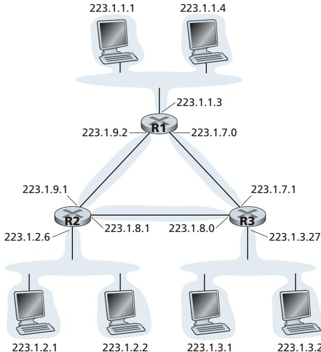
**Figure 4.17** ♦ Three routers interconnecting six subnets
