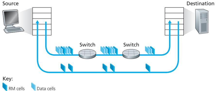
**Figure 3.50** ♦ Congestion-control framework for ATM ABR service
