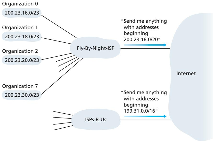
**Figure 4.18** ♦ Hierarchical addressing and route aggregation
