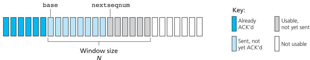
**Figure 3.19** ♦ Sender's view of sequence numbers in Go-Back-N
