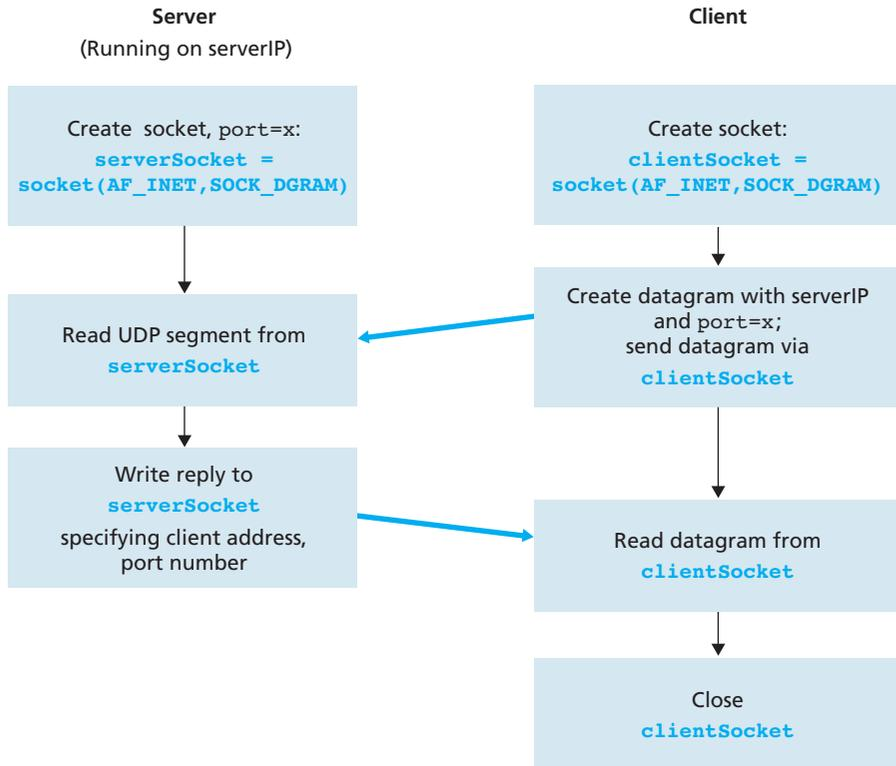
**Figure 2.28** ♦ The client-server application using UDP
