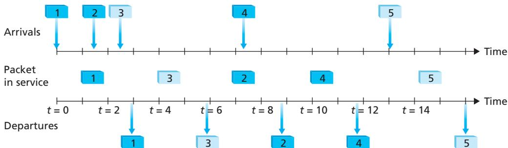
**Figure 7.21** ♦ Operation of the two-class round robin queue
