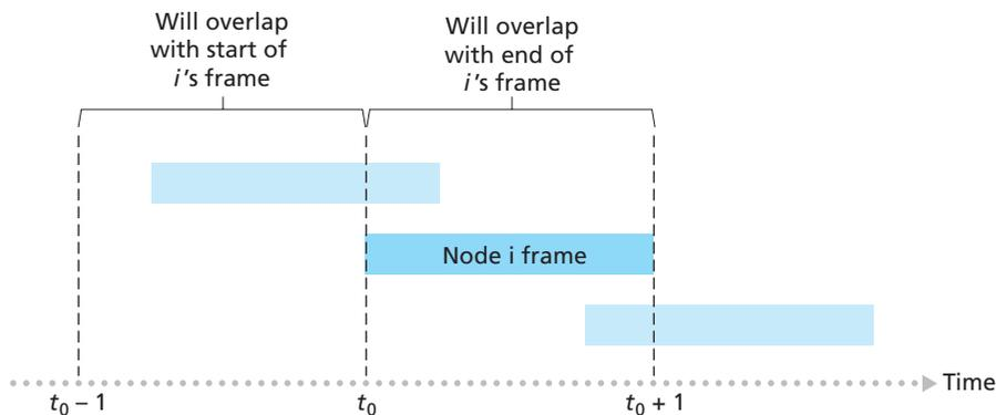
**Figure 5.11** ♦ Interfering transmissions in pure ALOHA
