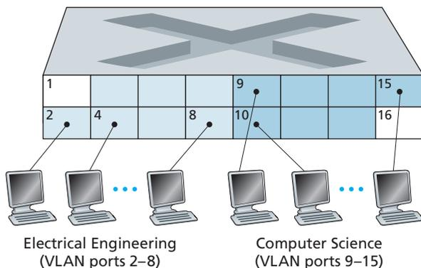
**Figure 5.25** ♦ A single switch with two configured VLANs
