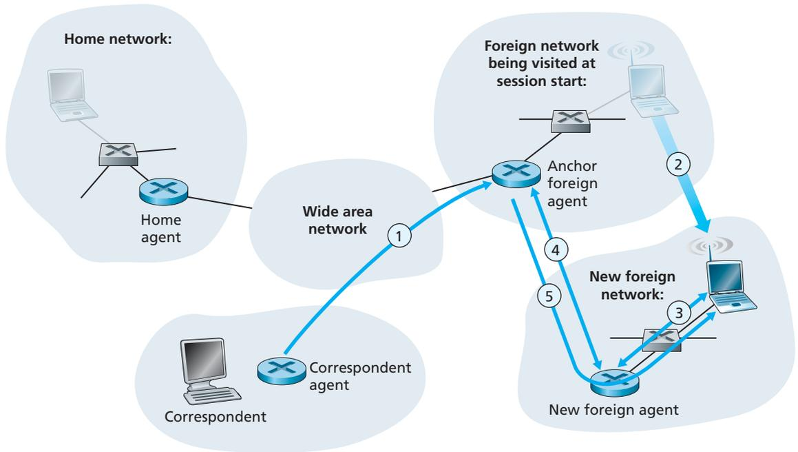
**Figure 6.26** ♦ Mobile transfer between networks with direct routing
