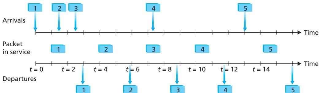
**Figure 7.18** ♦ The FIFO queue in operation
