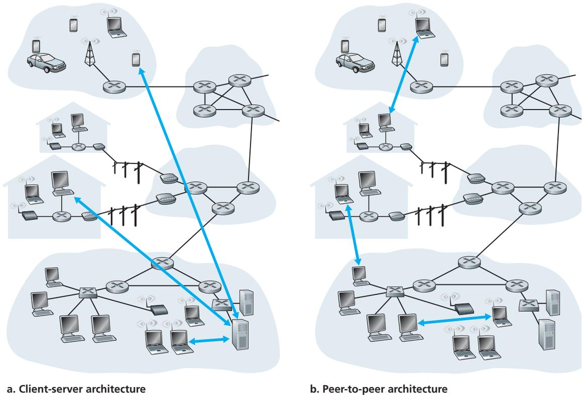
**Figure 2.2** ♦ (a) Client-server architecture; (b) P2P architecture
