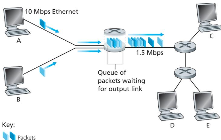
**Figure 1.12** ♦ Packet switching
