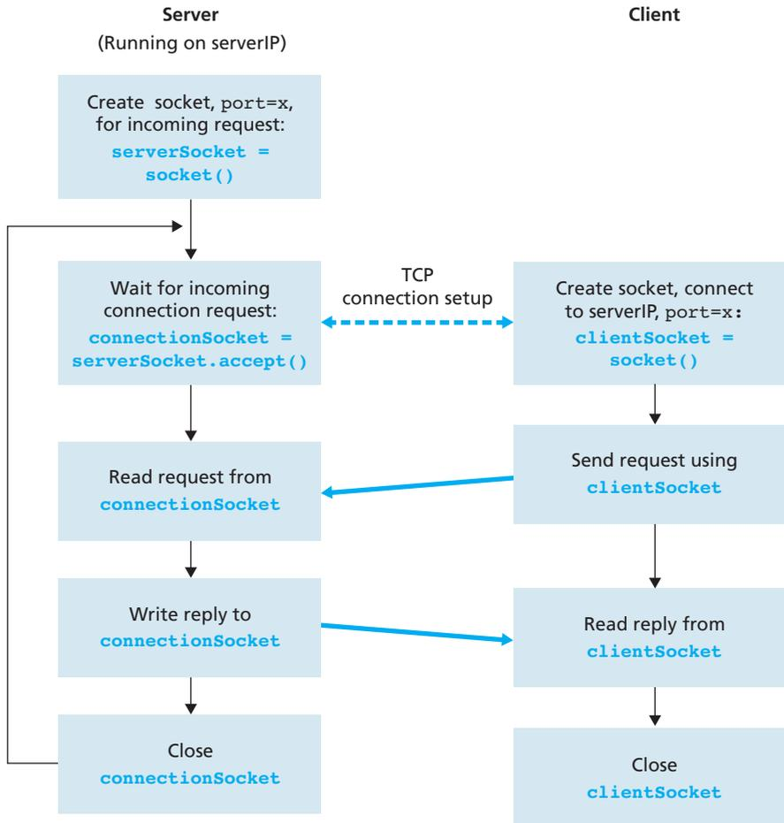
**Figure 2.30** ♦ The client-server application using TCP
