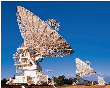
Incoming signals are reflected by the parabolic antenna to the receiver at the focus.
