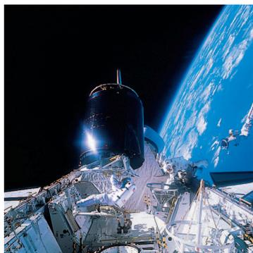
Astronauts use tools that are designed to limit forces that would impart unintended rotational motion to a satellite.
