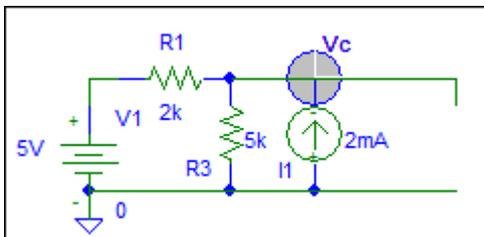
$$-2 + \frac{V_C}{R_3} + \frac{V_C - V_1}{R_1} = 0 \quad (13)$$
