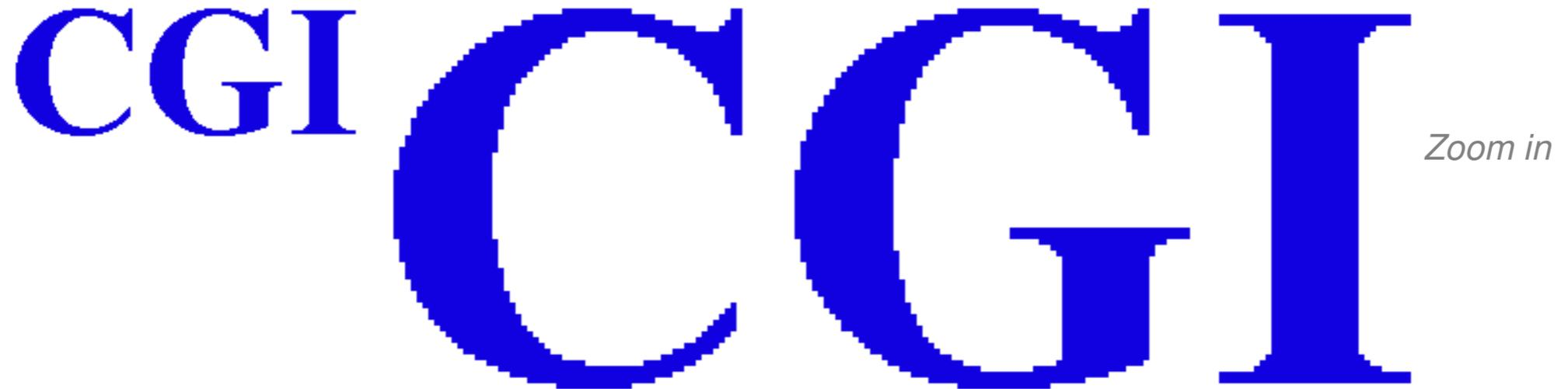
The image shows the text 'CGI' in a standard Times New Roman font. To its right, the same characters 'C', 'G', and 'I' are shown at a larger size, illustrating the 'staircase' effect where the edges of the letters are jagged and pixelated due to lack of antialiasing.
