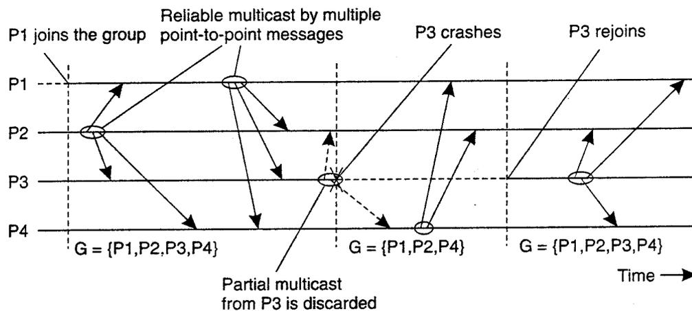
Figure 8-13. The principle of virtual synchronous multicast.
