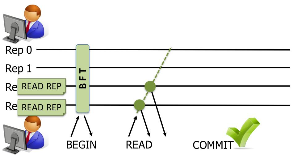
Reads from different clients striped to different replicas => reduced load on each server
