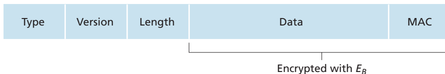
Figure 8.26 ♦ Record format for SSL
